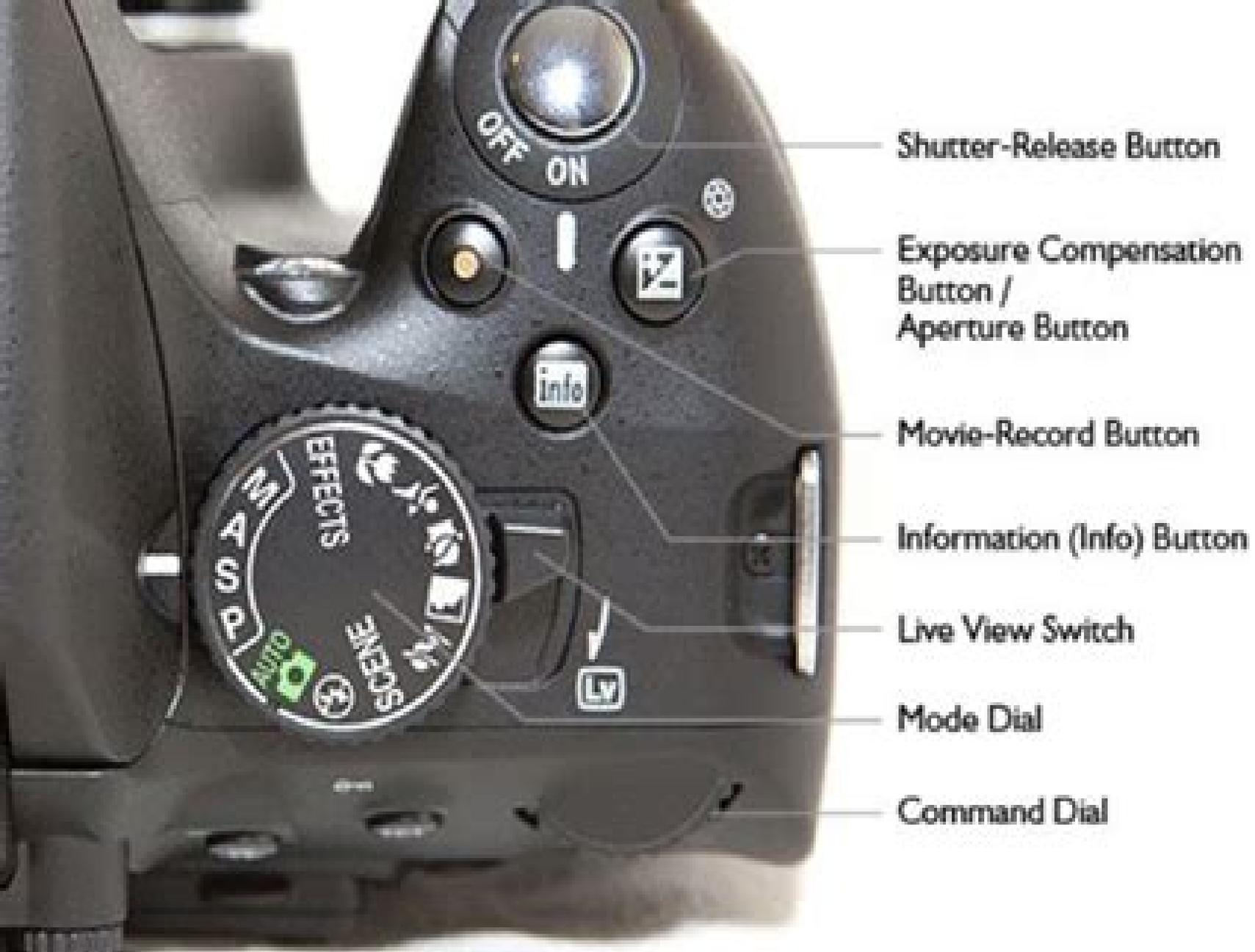
*Figure 2 - Controls on the top of the D5100*
