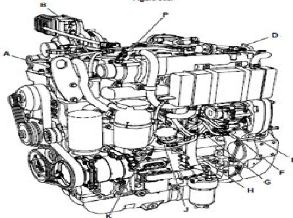
A Coolant temperature sensor (PIL 15-84)
