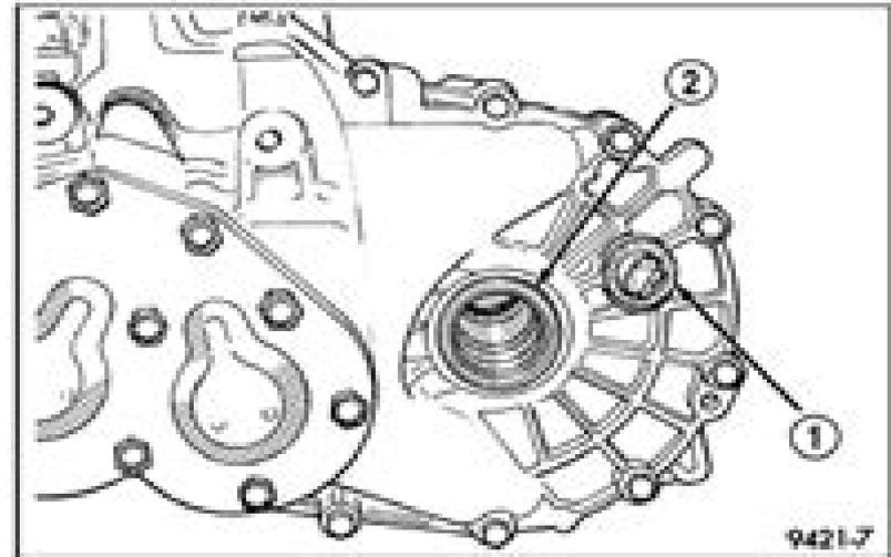
The transaxle drain plug (1) is located on the lower right side of the transaxle differential housing. Tighten drain plug to 14 N-m (120 in. lbs.).
